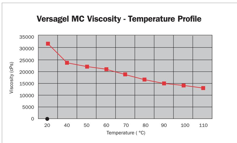
Like the other Versagel products, Versagel MC is shear thinning. However, the Versagel MC products are unique in that they exhibit minimal “stringiness” due to the short hydrocarbon chain structure of the base oil. This characteristic is desirable in certain applications where elasticity needs to be minimized. The graph shows how viscosity decreases as the temperature increases for Versagel MC 750.
