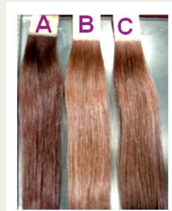
Fig. 3: Color wash fastness efficiency of ABIL® ME 45 MB – differences in color after 20 washing cycles
