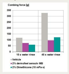
The conditioning performance and the lastingness of **dermofeel® sensolv MB** is comparable to Dimethicone 10 mPa·s.
