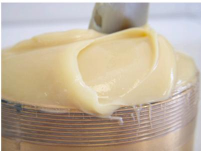
Beside the application in a wide range of manufacturing processes, LAVIOSA VISCOGEL™ are used as Thickeners for Clay Base Grease to give the desired rheological control to the lubricating system.
